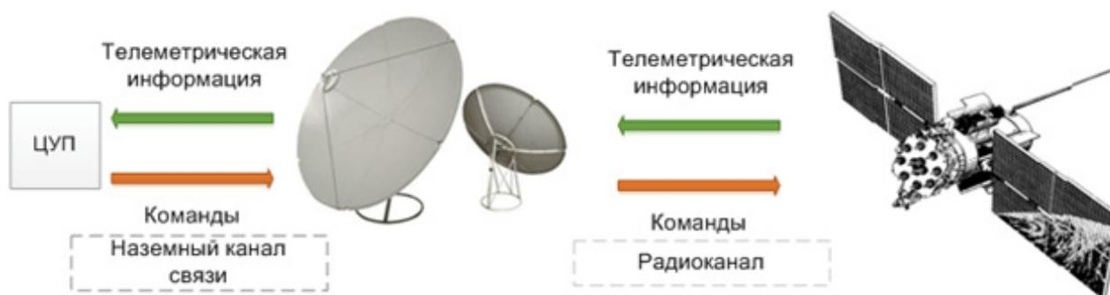
Fig. 1. Sending sequence of commands to CS
