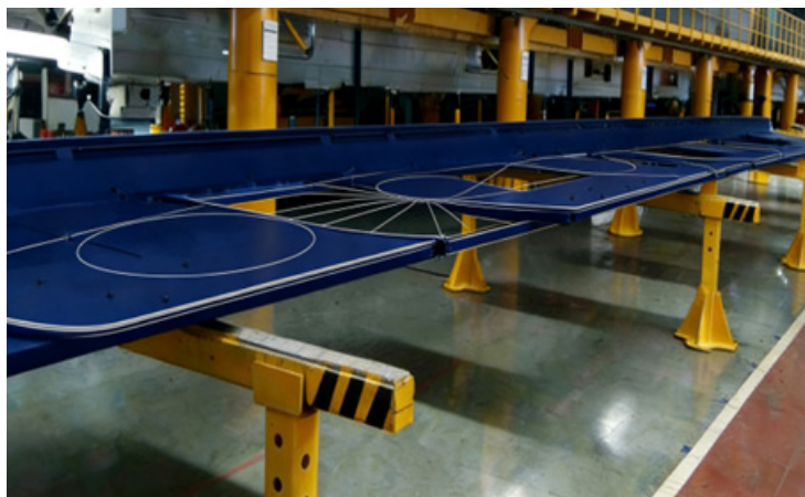
Fig. 3. Application of a universal adjustable support device
