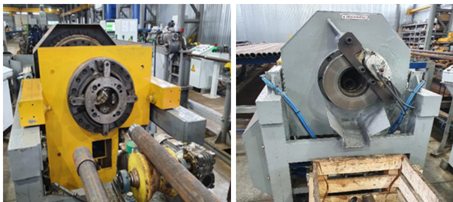
Fig. 3. Machine for unscrewing couplings (prototype)
