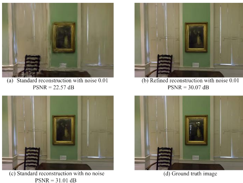
Fig. 2. Comparison of novel view synthesis with and without camera pose refinement at noise level 0.01. Standard 3DGS reconstruction with noisy camera poses results in significant quality degradation when compared to the same reconstruction without noise (c) and the ground truth (d). By applying our proposed in-training camera pose refinement, we achieve a reconstruction that closely resembles the ideal ground truth data
